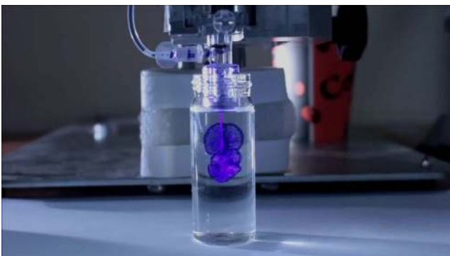
FIGURE 1 Multidirectional dispersion of the colored HA jet injected into polyacrylamide gel vial (Courtesy of PerfAction)
